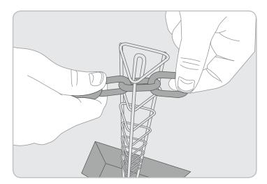
Thread the first link on the chain through the top section of the upright and position onto 1 the integrated hook. Continue by feeding the opposing end of the chain through the adjacent upright until the sag in the chain is approximately 100 mm below the horizontal then attach the intermediate link to the hook.
