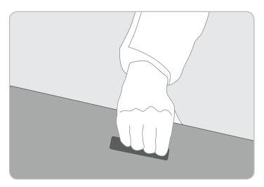
**1** The base weights are designed with a carrying handle and weigh 16.8 kg each. Refer to the Lifting Operations and Lifting Equipment Regulations 1998 (LOLER) for guidance on safe lifting and be certain to only lift what you are comfortable with.
