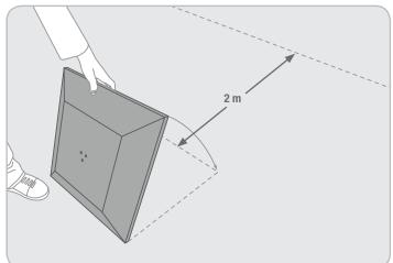
2 Measure 2 m from the hazard whilst being sure to stay at a safe distance from the edge. Remaining within the safe zone, position the first base at this point, placing it down outwards, away from the body as shown, with the D-marc logo facing away from the hazard. NB: When installing the system onto a single ply roofing membrane, consult the relevant manufacturer for advice.
