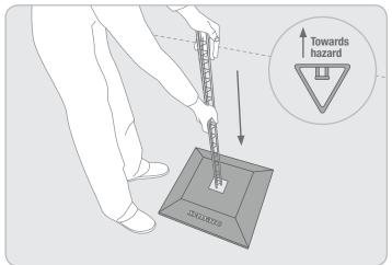
Insert the D-marc 105 upright into base ensuring the integrated hook for the chain is on the side facing the hazard. The upright base plate must fit flush into the weighted base.
