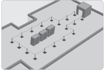
Thread the rest of the chain through the D-marc 105 uprights until reaching the final 8 Thread the rest of the chain unrough the D-main from upnging that is a solid chain link supplied multiple lengths of chain be required join each by using the split chain link supplied.
