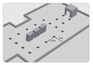
**3** Lay the rest of the bases in the same way along the edge of the demarcation zone at regular distances of no more than 3 m apart. Should a corner post be required the bases may be positioned at 90° degrees from each other or even at an acute angle.
